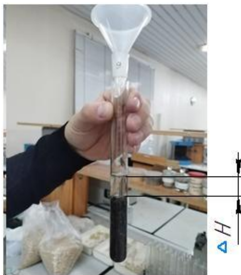
Figure 3 - Measurement of volume change after adding fertilizer sample
