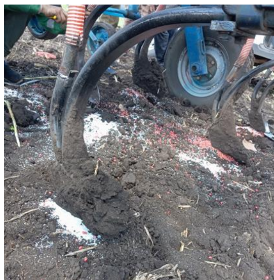
Figure 6 – Soil adhesion to the surface of rippers (soil moisture \phi=29.8\% )
