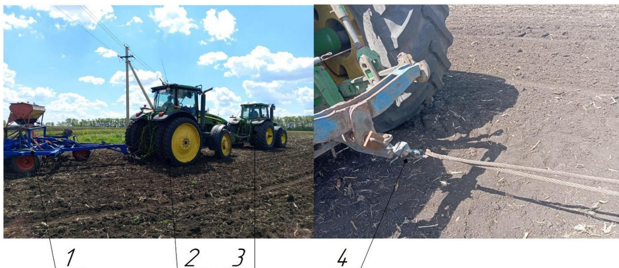
1 – cultivator; 2 – tractor-tractor John Deer 7000; 3 – aggregated tractor John Deer 7000; 4 – load cell
